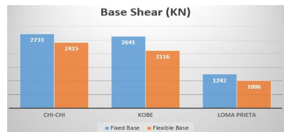
Figure 9. Base shear outputs of numerical modelling for the Fixed base and the Flexible base models
