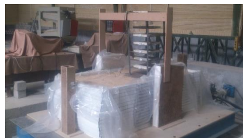
Figure 7. LSB and soil-structure system
