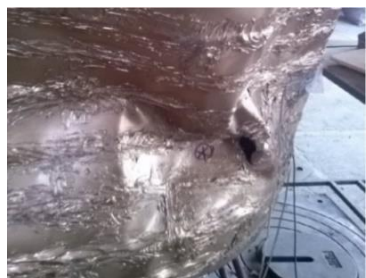
Figure 11. Weld line failure of the experimental Spec2
