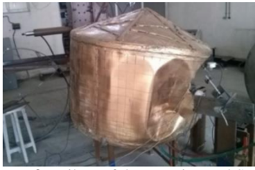
Figure 9. Failure of the experimental Spec1
