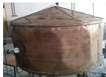
Figure 8. Full buckling of Spec1 and instability threshold
