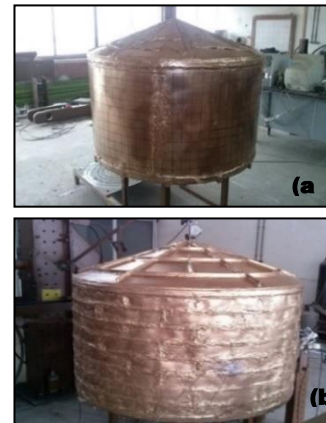
Figure 5. Experimental specimens: (a) Spec1 in an integrated form (b) Spec2 in panelized form
