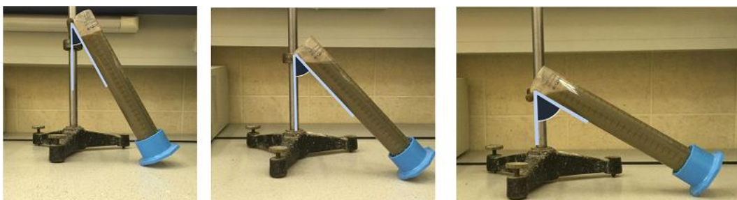
Figure 1. Cement slurry placement at different angles of 30°, 45° and 60° with respect to the vertical plane
