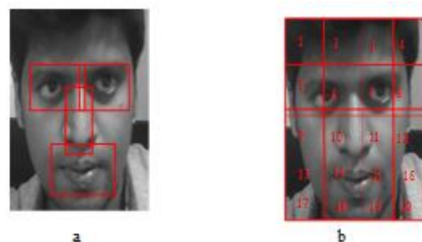
Figure 8. (a) For face recognition, a face image is roughly divided into four semantic patches. (b) For identity recognition, a face image is divided into twenty semantic square regions
