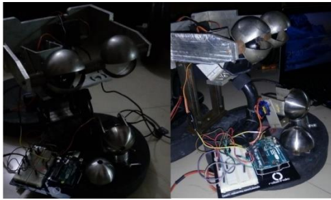
Figure 1. Fabricated model of a humanoid vision system with camera holding structure and connecting plate which support pan and tilt mechanism. The Camera is covered by 180deg eyeball
