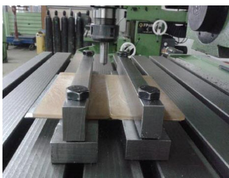
Figure 5. Fixture, clamps and specimens mounted on the milling machines
