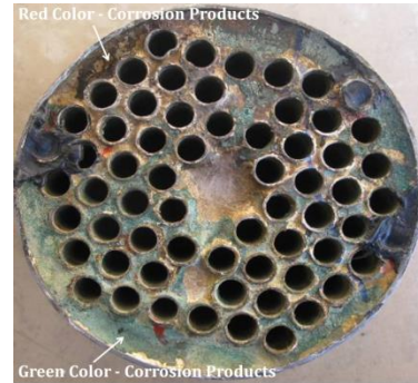
Figure 4. Red color and green color - corrosion products on the tube sheet
