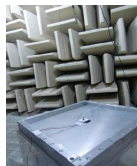
Figure 11. Sound isolation tests in the anechoic chamber
