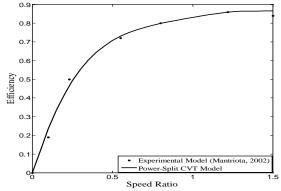
Figure 5. The comparison of the power-split CVT model and experimental model [22]
