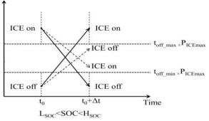
**Figure 3.** Schematic of the method proposed to reduce the start/stop frequency of the ICE and the EM
