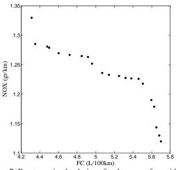
**Figure 9.** Pareto-optimal solutions for the case of considering FC and NOX as the objectives
