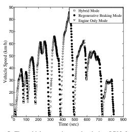
Figure 8. The vehicle operation modes during SC03 for the case of using the unmodified control strategy
