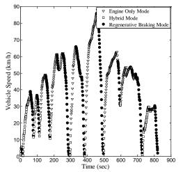
Figure 7. The vehicle operation modes during SC03 for the case of using the modified control strategy
