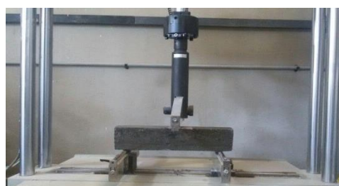
Figure 3. concrete beam under third point loading for flexural strength test
