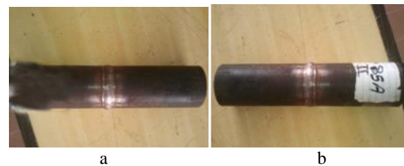
Figure1. Pipe after welding by a) SMAW and b) GTAW techniques
