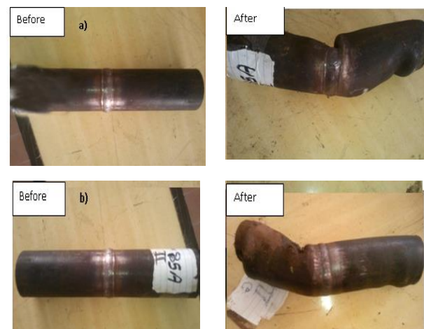
Figure 2. Steel pipes a) SMAW b) GATW welding techniques
