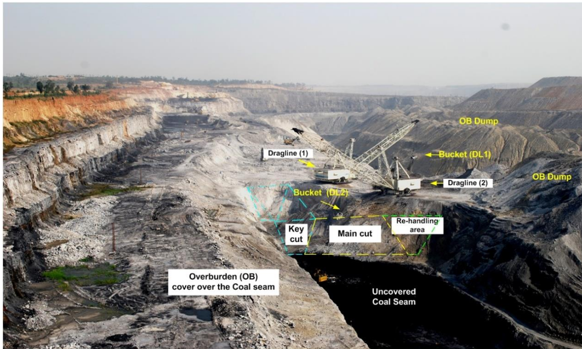
Figure 7. Draglines in horizontal tandem operation
