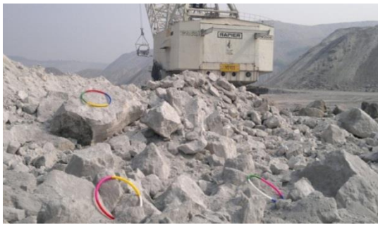
Figure 8. Collar oversize fragmentation at the key-cut
