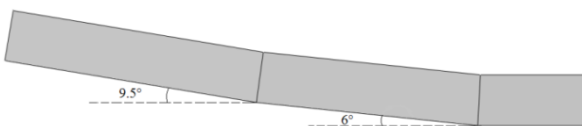
Figure 4. 2D view of die land and die inlets of hammer in RFP
