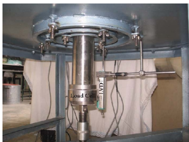
Figure 12. Ttrapdoors, load cell and displacement gauge
