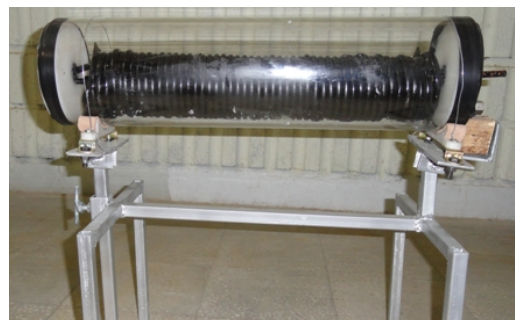
Figure 1. Cylindrical solar collector with copper helical tube receiver.
