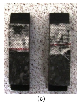
Figure 5. (a) Preparation process of specimen, (b) schematic of specimen and (c) non adhering film as a pre crack
