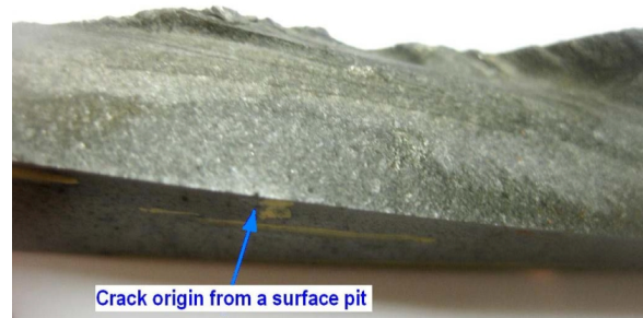
Figure 9. A view of the fractured bled surface with a pit on the pressure side.
