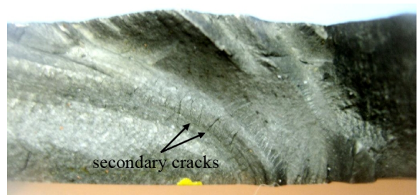
Figure 10. Presence of secondary cracks near the final fracture zone (high stresses)
