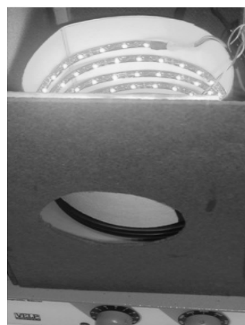
Figure 6. Location of the LED SMD extensions
