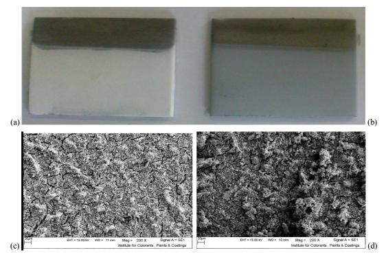
Figure 4. Macroimages of as deposited thick films: (a) HA and (b) HA-5%wt CNT coatings. Also shown SEM images of (c) HA, and (d) HA+CNT coatings.
