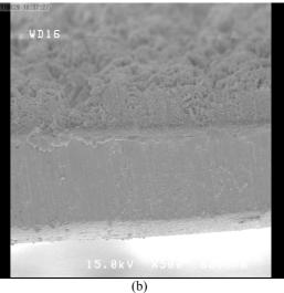
**Figure 6.** SEM images from cross section of (a) HA and (b) HA-5% wt CNT coating deposited at 100 V and 3 min (500X).
