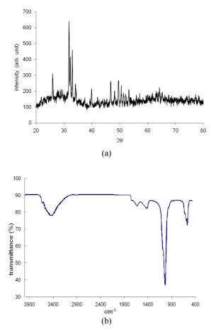
**Figure 2**. (a) XRD and (b) FTIR specra of the synthesized HA powder after calcination at 900 °C for 2 h
