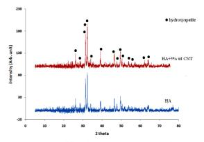
**Figure 7.** X-ray diffraction patterns of HA and HA-5%wt CNT coatings after sintering at 850 °C for 2 hr in argon atmosphere. All the peaks correspond to hydroxyapatite composition (JCPDS 01-070-0795)
