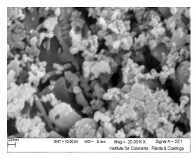
Figure 3. SEM micrograph of the as- calcined HA powder
