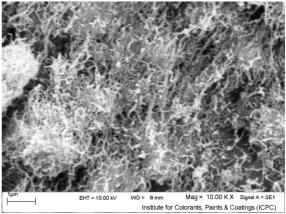
Figure 1. SEM images of the as-received CNT
