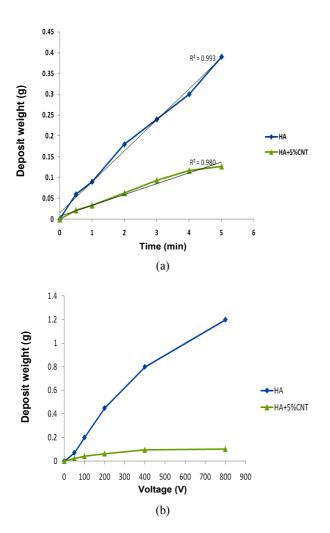
**Figure 5.** Variation of deposit weight by (a) deposition time and (b) electric field voltage for HA and HA-5%wt CNT coatings. The deposition area and the electrode distance are the same for all the samples ( $4 \times 3 \text{ cm}2$  and 3 cm, respectively).
