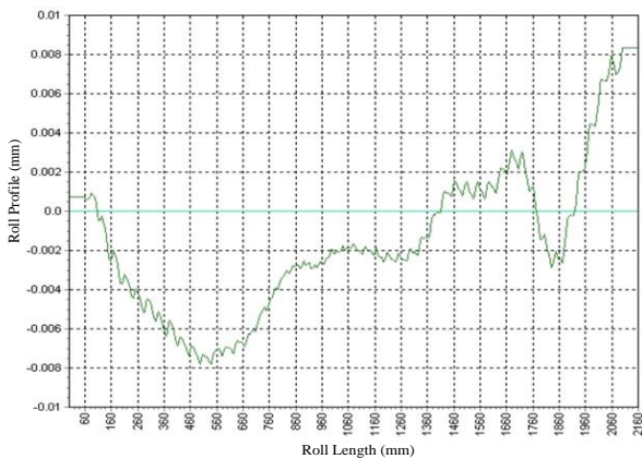
Figure 5. Measured roll profile before one of the rolling schedules for stand No. 6.
