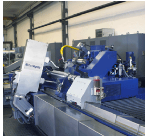
Figure 4. Herkules WS450 machine for measuring the rolls wearing crown
