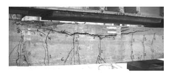
Figure 9. Flexural failure of control beam AH0.
