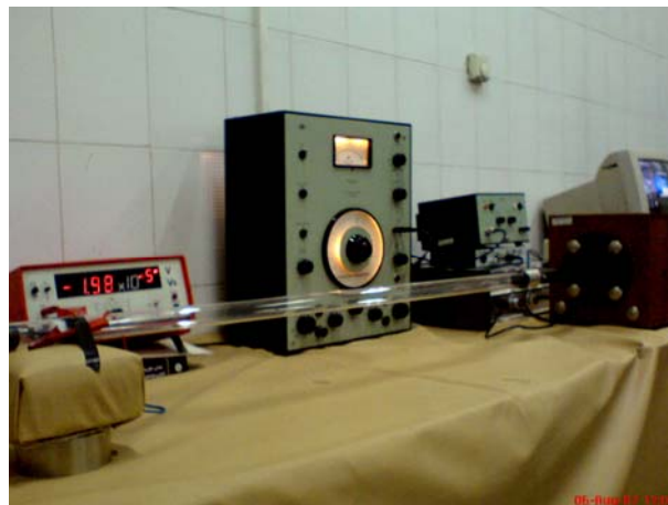
Figure 5. Experimental set-up of thermoacoustic refrigerator.
