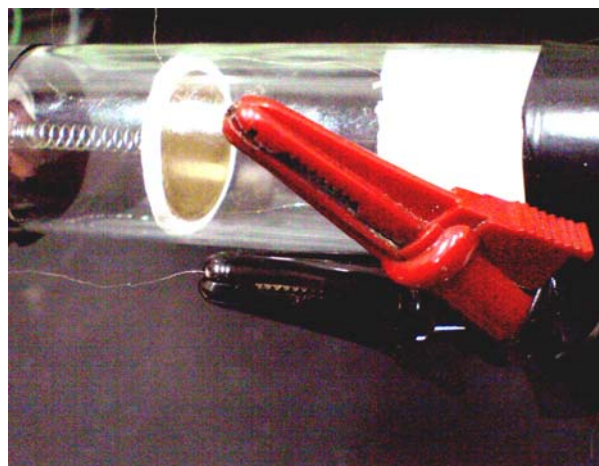
Figure 6. An adjustable coupled mechanical resonator that we added to the end of the resonator tube of thermoacoustic refrigerator. It consists of a screw connected to a nonlinear spring at the end of the tube. The other end of the spring is connected to a metal plate with electrical nonconductor perimeter.
