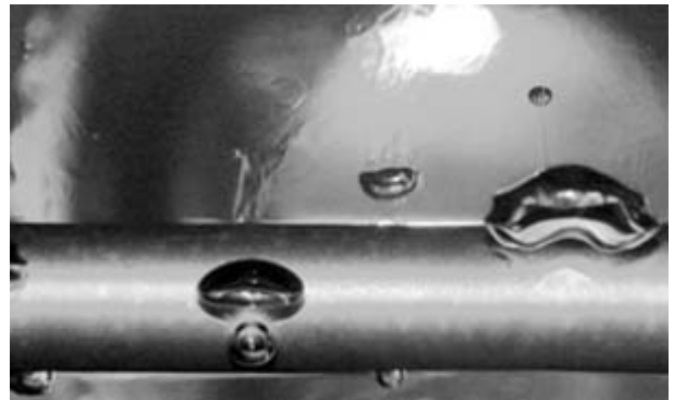
Figure 13. The appearance of heat transfer surface during boiling of water/Diethanolamine mixture [ q = 42 \text{ kW.m}^{-2} , X (Acetone) = 0.5].
