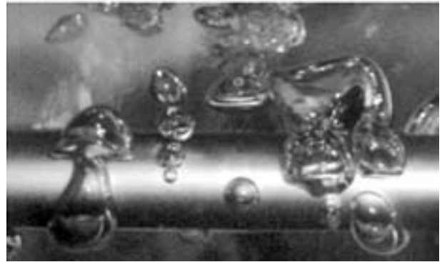
Figure 12. The appearance of heat transfer surface during boiling of water/Monoethanolamine mixture [ q = 90 \text{ kW.m}^{-2} , X (Acetone) = 0.5].
