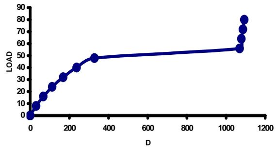
Figure 10. Static path for truss with 22 members.
