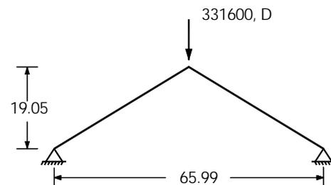
Figure 1. Truss with two members.
