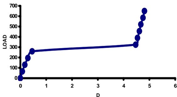
Figure 8. Static path for truss with 24 members.
