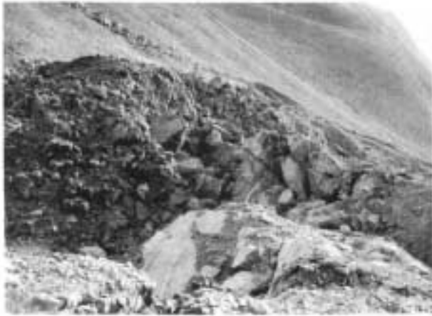
Figure 2. One typical of bad explosion " Too much oversize".
