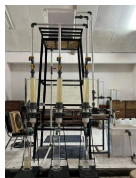
Figure 2. Equipment for the performance and leaching tests of PMF specimens
