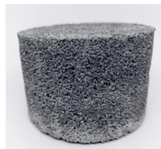
Figure 1. Pervious mortar filter with the dimension of 8.2 cm (d, diameter) x 5 cm (h, or thickness), made of sand with a grain size of 0.6–0.85 mm and a sand-to-cement ratio (M) of 4
