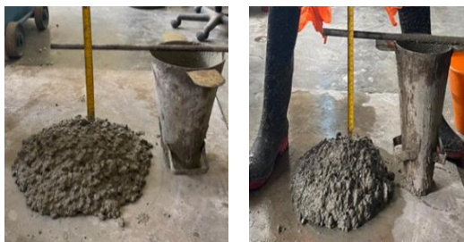
Figure 6. Visual observations of slump tests in fresh concrete
