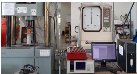
Figure 3. Concrete specimen test setup
