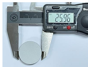
Figure 12. Appearance of pure Al-coated specimen carried out at Impact-Innovations GmbH in Germany
