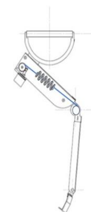
Figure 3. Form of the elastic element inside hip link of orthosis
