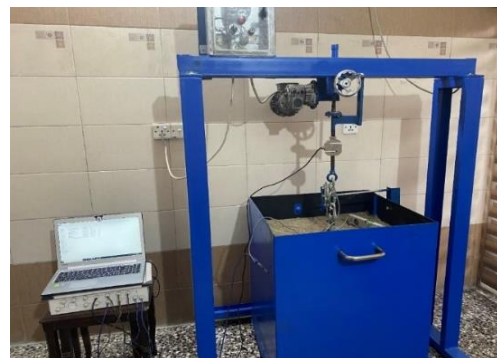
Figure 2. Under-reamed pile test
