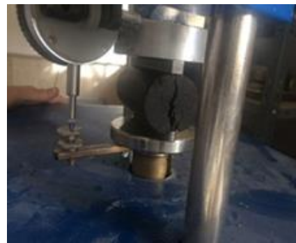
Figure 4. Preparation and loading of organic soil samples for indirect tensile testing
