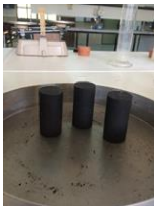
Figure 3. Cylindrical specimen made of organic soil
