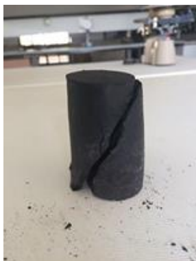
Figure 8. Plane failure of the specimens in the unconfined compression test
