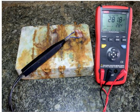
Figure 7. Schematics of corrosion monitoring of rebars in reinforced concrete by a LCR meter
