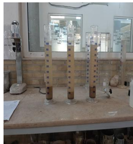
Figure 3. Particle size distribution (hydrometer analysis)
