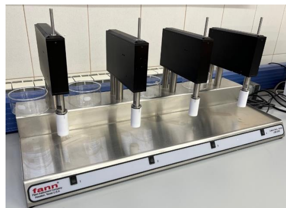
Figure 3. Linear clay swelling tester LSM 2100 (compiled by the authors)
