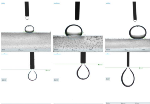
Figure 4. View of lying and hanging droplets from which the edge wetting angle and interfacial tension forces are determined (compiled by the authors)
