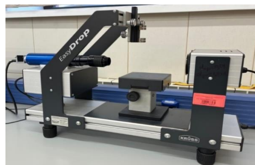
Figure 1. Device for measuring the edge angle of wetting Easydrop (compiled by the authors)
