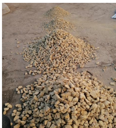
Figure 2. Preparing the CCB for lightweight aggregate
