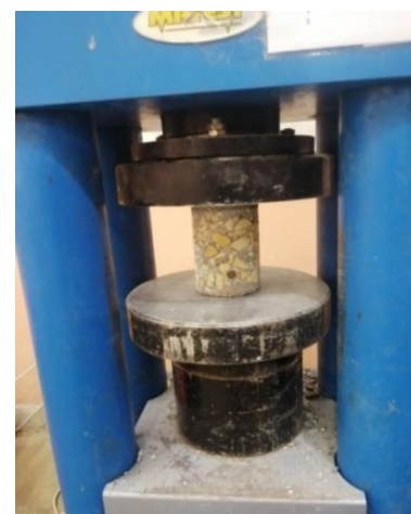
Figure 5. LWC cores under compression test
