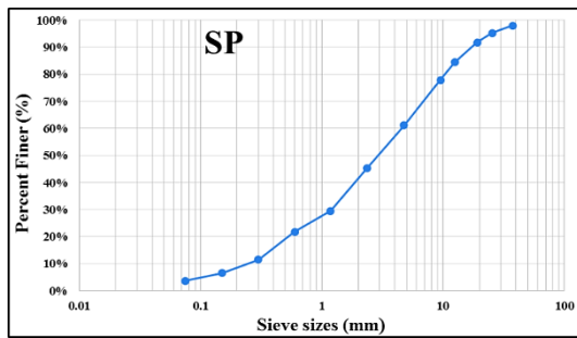
Figure 4. The gradation curves of coarse-grained materials used in the layers of road projects
