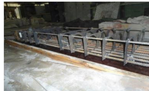
Figure 5. Preparation and lying the bubbles on the right side of the specimen
