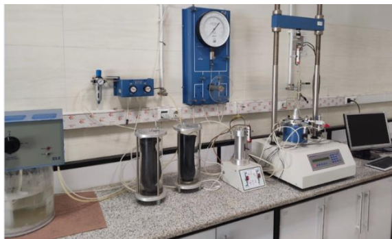
Figure 17. Used triaxial device
