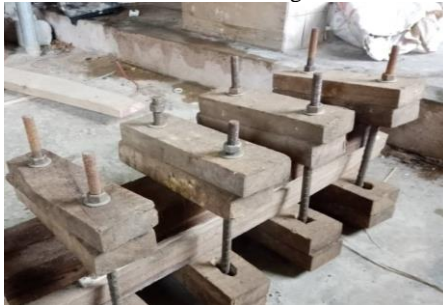
Plate 2. Improved clamping system for pressure application
