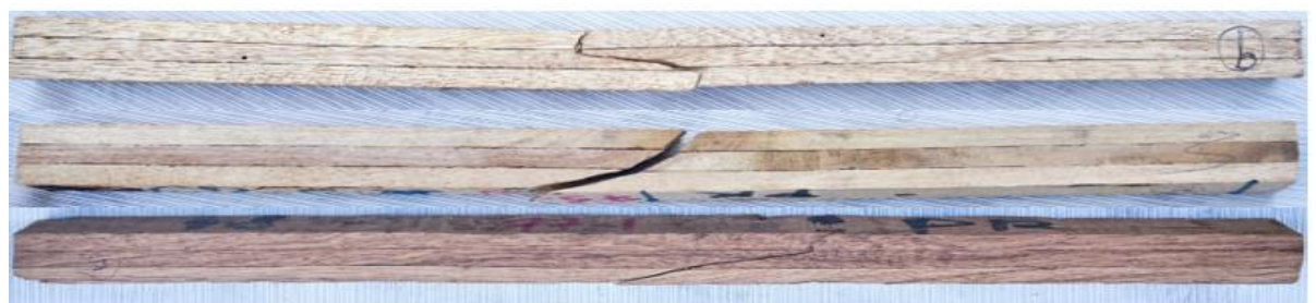
Plate 5. Cross grain tension failure in glulam beams
