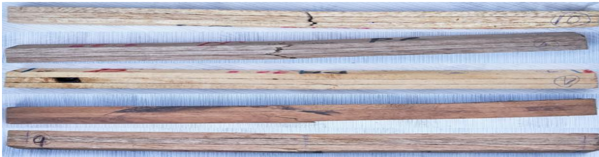
Plate 4. Fracture form of glulam beams from up to down: Afara, Akomu, Gmelina, Iroko and Omo cedar wood species
