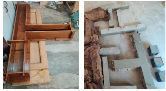
(a) Prepared Plywood Mould for casting (b) Prepared specimen during casting and curing Figure 2. Preparation of mould and specimen
