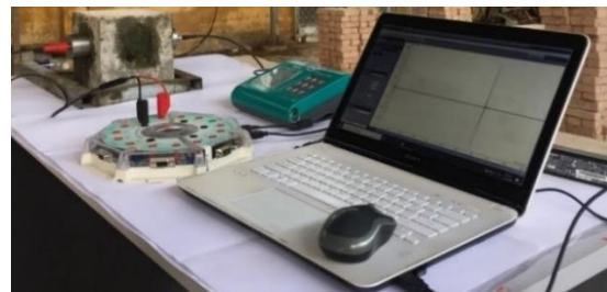
Figure 7. Device connection diagram to receive wave signal
