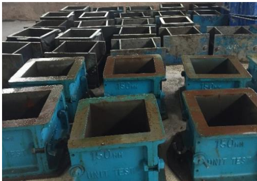
Figure 3. Mold for making concrete samples
