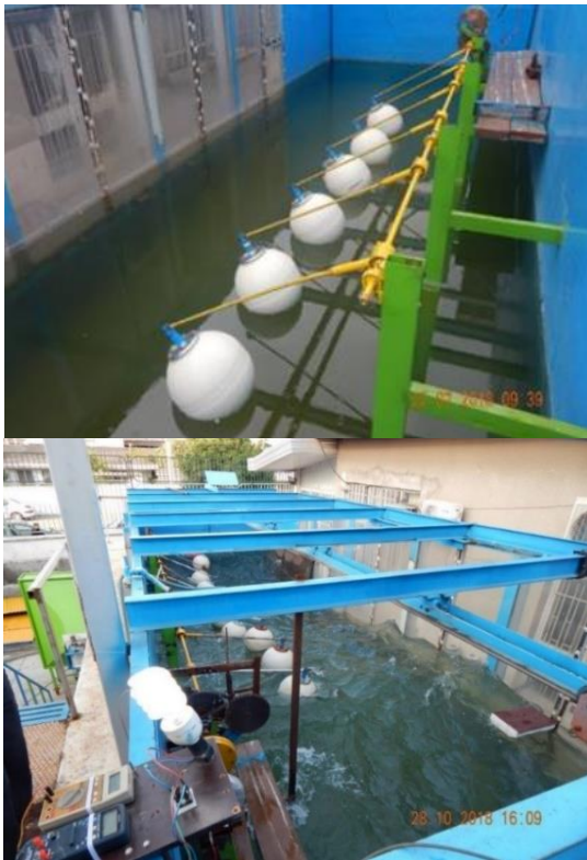
Figure 2. Centipede WEC constructed and tested in BNUT, at Sea-based Energy Research group test rig by mechanical PTO system in 6 and 10 buoy arrays [20]
