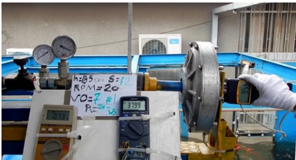
Figure 8. hydraulic and electric output data measurement equipment
