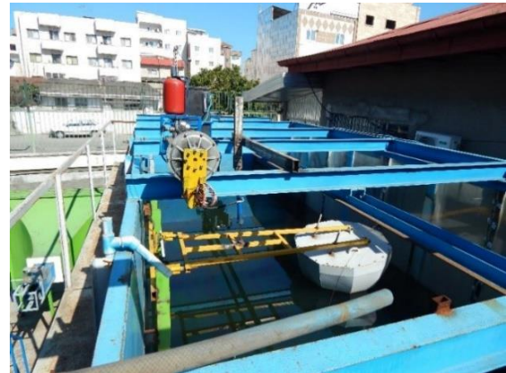
Figure 4. installation mode of centipede WEC in the wave tank
