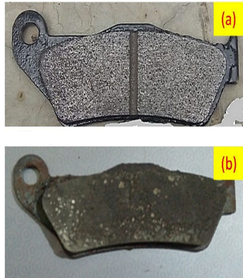
Figure 10. Brake pads (a) Commercial (b) Newly developed
