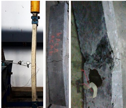
Figure 13. RPG column: (a) Buckling failure (b) tensile cracks (c) Progressive compression failure
