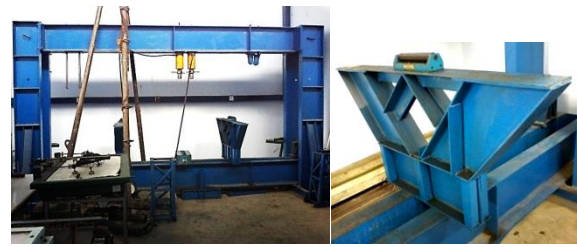
Figure 6. (a) Loading frame; (b) dial gauge support
