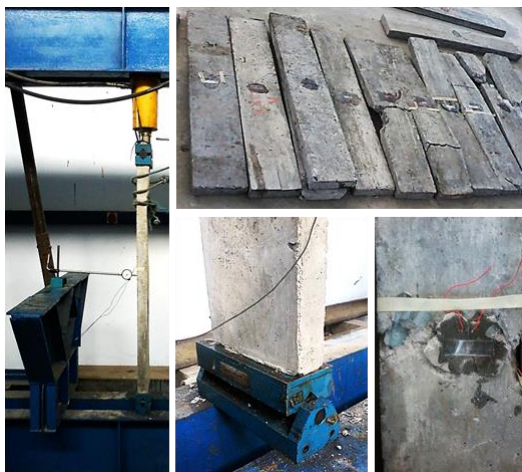
Figure 14. (a) Loading begin at UHP column before buckling (b) Behaviour of specimen collapse (c) joint support (d) local compressive failure
