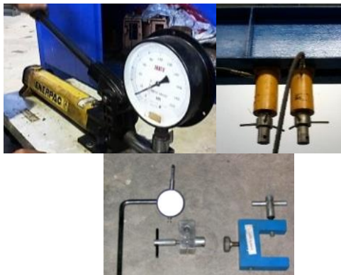
Figure 5. (a). Hand pump (b) hydraulic jack, (c) Dial gauge, dial holder and clamp
