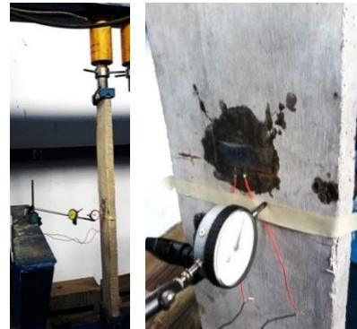
Figure 11. (a) CWG as column without glass due to axial load before buckling occurs (b) position of the glassless column strain gauge
