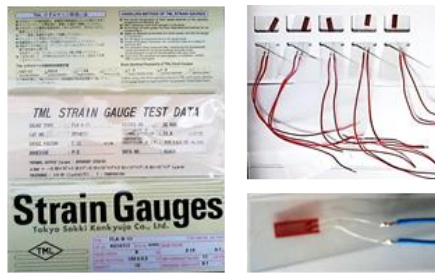
Figure 9. Strain gauge with a resistance of 120 ± 0.3 Ω
