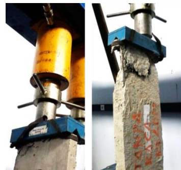
Figure 12. (a) local collapse on the RPG column support (b) upper RPG column spalling at peak load
