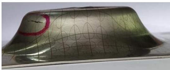
Figure 5. Component formed with 65° wall angle whereas it is marginal increase in case of minor
