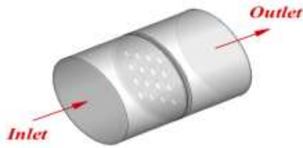
Figure 1. Overview of the 16-hole orifice and the fluid passing through it
