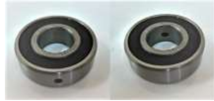
Figure 2. Defective bearings with created holes of 2-mm diameter on the inner race and outer race
