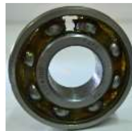
Figure 4. Defective bearing with a rupture in the chain
