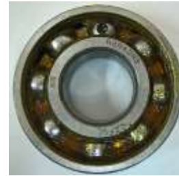
Figure 3. Defective bearing with a created hole of 2-mm diameter on a ball
