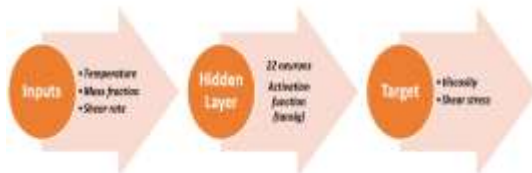
Figure 3. Optimal neural network structure
