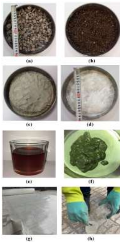
Figure 1. Used material a: Coarse aggregates b: Fine aggregates c: Cement d: GF e: Superplasticizer f: FSCG g: GFRP plates h: Paste
