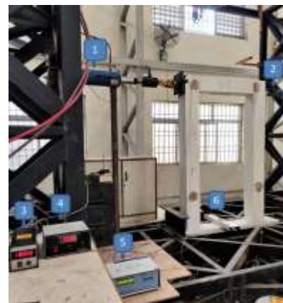
(1) Hydraulic jack 200 kN capacity, (2) LVDT, (3) Deflection indicator, (4) Load indicator, (5) Multi-channel data logger, and (6) Strain gauges on the surface
