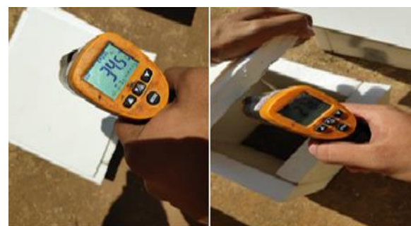
Figure 5. Temperature testing inside and outside of tile
